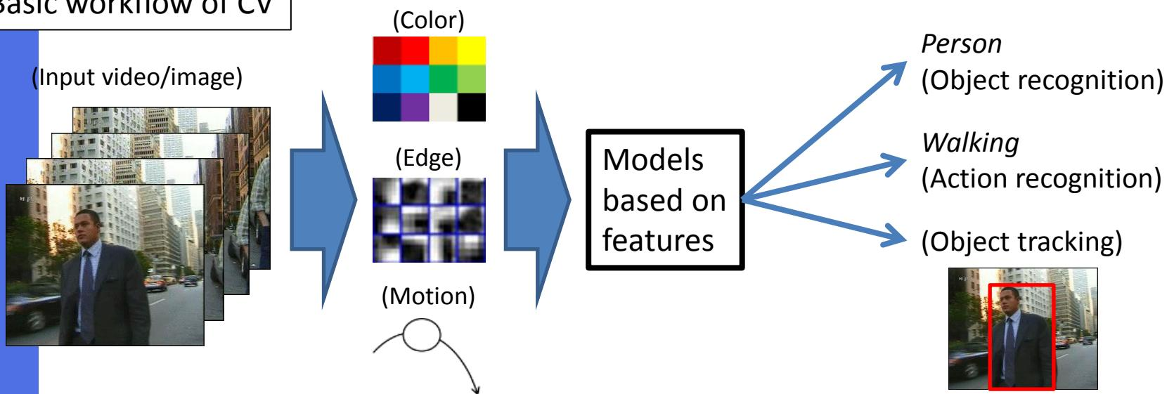
Many functions in this workflow have been implemented in OpenCV!
